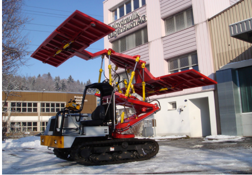
Mobile positioning system
